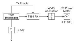
Figure 3.1 T889 Test Equipment Set-up
